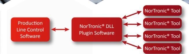
NorTronic® DLL (Dynamic Link Library) plugin enables NorTronic® 868 MHz and 915 MHz version tools to be interfaced to a customer's existing production line control software. DLL is not compatible with Bluetooth® versions. Contact Norbar for more details.
