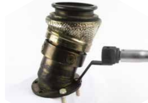
Special spanner fitting for Fuel Cooled Oil Cooler (FCOC) – Panavia Tornado
