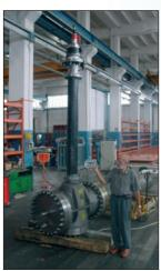
Ball valve actuation using PT13
