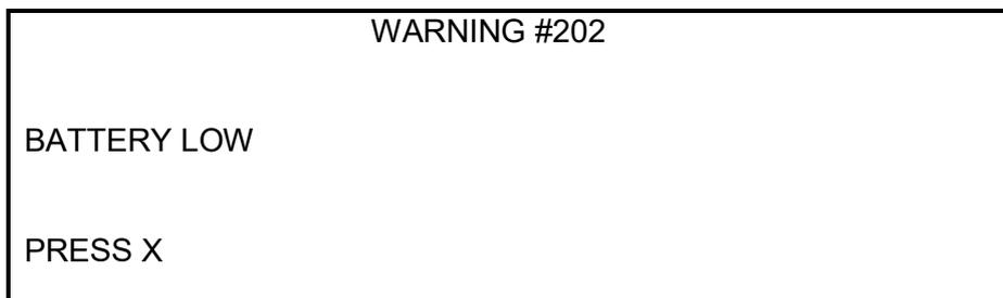
When battery is flat the TTL-HE must be turned off or recharged. The following is displayed:
