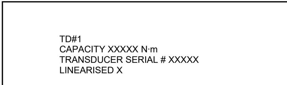
**NOTE:** If the word 'LINEARISED' and direction arrows appear on this screen then the TTL-HE is using a second order polynomial to linearise the transducer.
