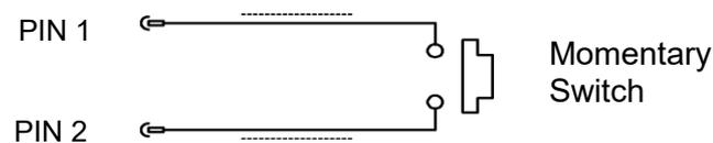
The switch must remain active for at least 200 mS. Screened cable is recommended.
