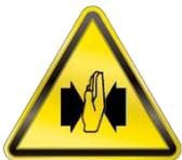
There is a risk of crushing between the reaction bar and work piece.
