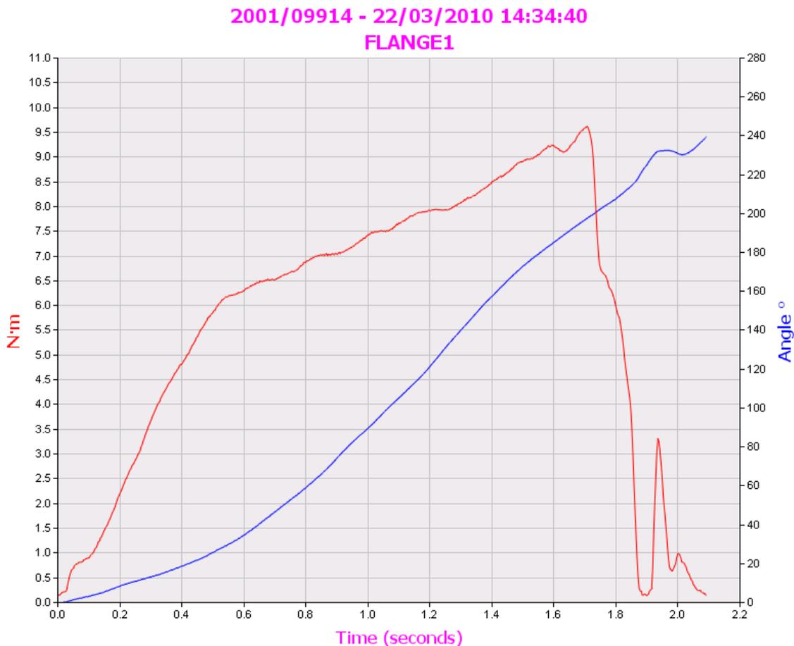
Graphs taken and saved on the T-Box XL™ can be sent to TDMS as Torque vs Time, or Torque & Angle vs Time.
