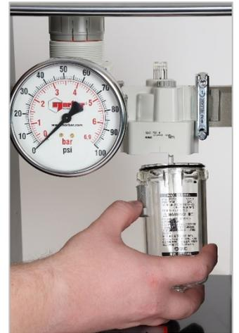
**FIGURE 6 – Lubricator Bowl Replacement**
