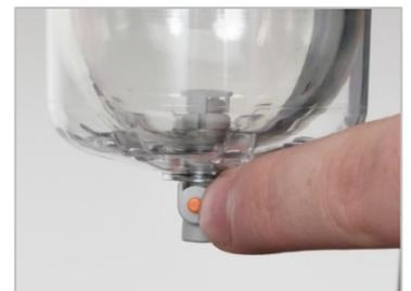
**FIGURE 7 – Draining Condensate**
