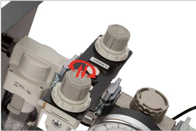
**FIGURE 3** – Front adjuster for “TORQUE 1”.
