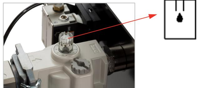
**FIGURE 5** – Lubricator Flow
