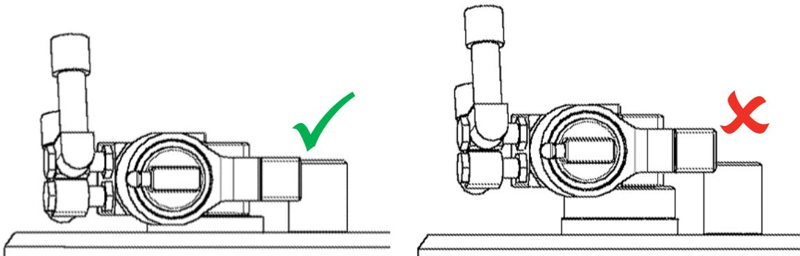
**IMPORTANT: ALWAYS REACT AS CLOSE TO BASE AS POSSIBLE. DON'T REACT AT TIP OF REACTION POST.**
