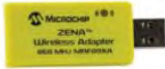
Alternatively plug in the Wireless adapter (part # 39671 - 868 MHz or part # 39672 - 915 MHz) into a USB port on your PC.
