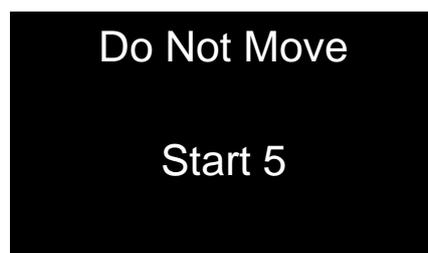
5 second countdown to the gyroscope drift calculation.
