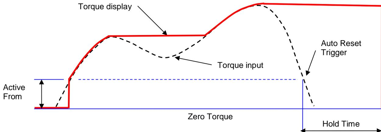
When torque is applied, the NorTronic® will track the torque input until it has exceeded the **Active From** setting (See page 50) and then enters into peak mode for both Torque & Angle.
