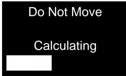
This screen is displayed during the gyroscope drift calculation.
