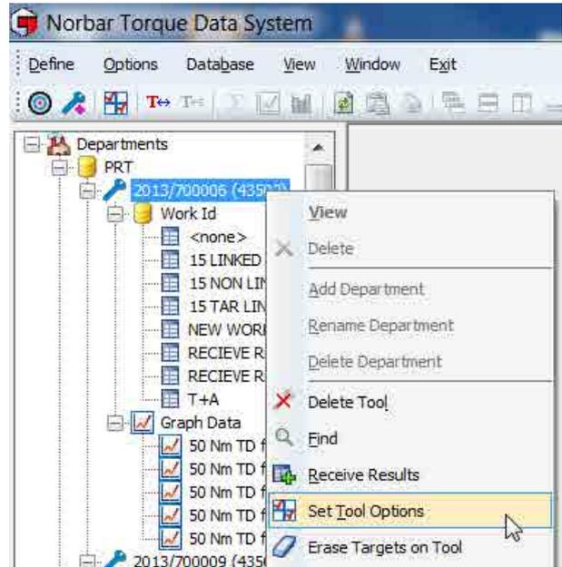
NorTronic® *Tool - set up* includes: *Limits, Units, Time & Date, Sleep, Angle Display, Auto Zero, Active From, Vibrate, Wireless, Auto Reset, Inverse Display, Torque Centres and Multiplier.*
