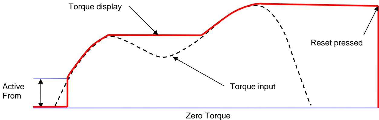
When torque is applied, the NorTronic® will track the torque input until it has exceeded the **Active From** setting (See page 20) and then enters into peak mode for torque and angle.
