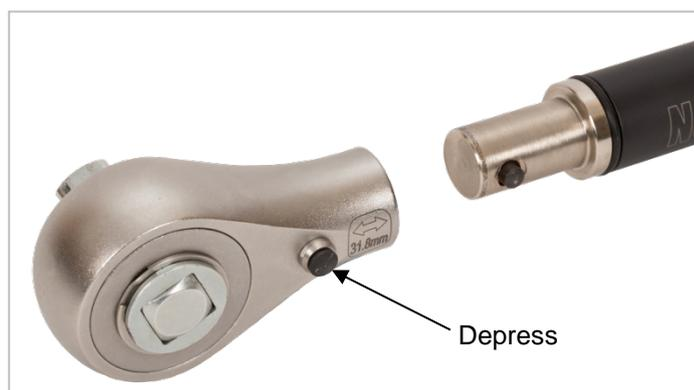
**NOTE:** All NorTronic® tools are Torque Handles with a 16 mm spigot. Should you wish to change to a different spanner end fitting, depress the plunger on the ratchet head and pull to release.
