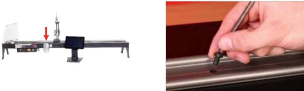
**FIGURE 21 – Removing Button Head Cap Screw**
