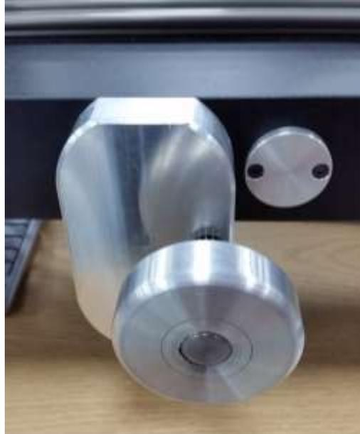
Use the Manual I/P Drive Gear Adaptor to achieve the correct value on the torque tool.
