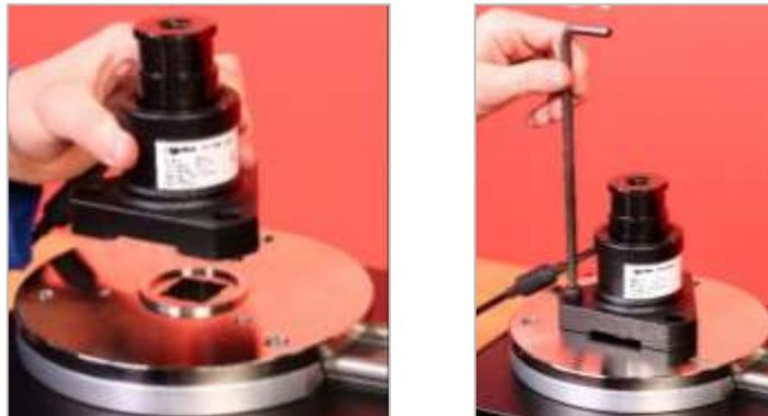
**FIGURE 14 – Fitting an FMT Transducer**
