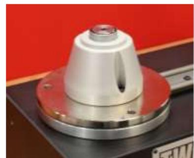
Place support over transducer and secure to TWC with socket cap screws provided.
