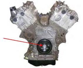
Crankshaft pulley bolt
